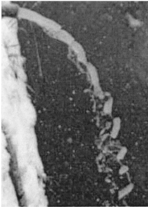
Fig. 6 High ice-fraction column flow at a pipeline outlet
